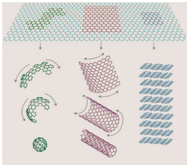
Graphene as a building block for carbon structures: (1) Bucky Balls (2) Nanotubes (3) Graphite
